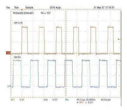
Figure 5-4. TPS54383EVM Switching Waveforms  $V_{IN}$  = 12 V,  $I_{OUT}$  = 2 A Ch1: TP9 (SW1), Ch2: TP12 (SW2) 5.5 Control Loop Bode Plot (low line,  $V_{IN}$  = 8 V)
