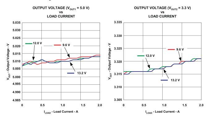
Figure 5-2. TPS54383EVM Output Voltage verse Load Current  $V_{IN}$  =9.6-13.2 V,  $V_{OUT1}$  = 5.0 V  $I_{OUT1}$  = 0-2 A,  $V_{OUT2}$  = 3.3 V  $I_{OUT2}$  = 0-2 A
