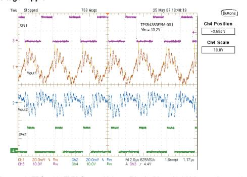
Figure 5-3. TPS54383EVM Output Voltage Ripple ( $V_{IN}$  = 13.2 V,  $I_{OUT1}$  =  $I_{OUT2}$  = 2 A)
