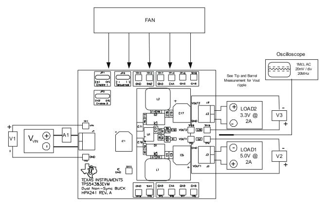
Figure 4-1. TPS54383EVM Recommended Test Set-Up
