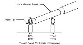
Figure 4-2. Tip and Barrel Measurement Technique (output ripple measurement using TP3 and TP4 or **TP18 and TP19**)
