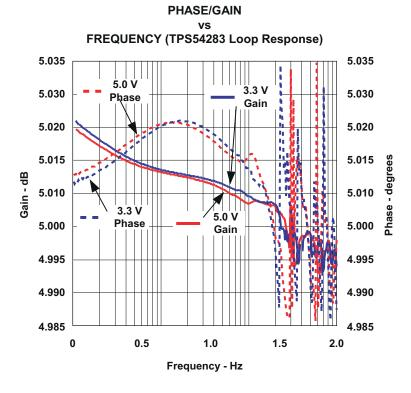
Figure 5-5. TPS54383EVM Gain and Phase vs Frequency
