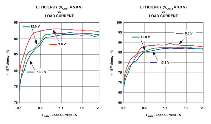
Figure 5-1. TPS54383EVM Efficiency verse Load Current  $V_{IN}$  =9.6-13.2 V,  $V_{OUT1}$  = 5.0 V  $I_{OUT1}$  = 0-2 A,  $V_{OUT2}$  = 3.3 V  $I_{OUT2}$  = 0-2 A
