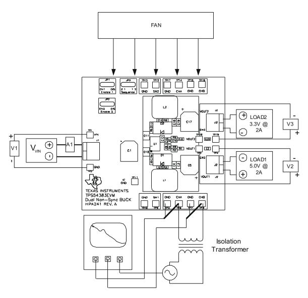
Figure 4-3. Control Loop Measurement Setup
