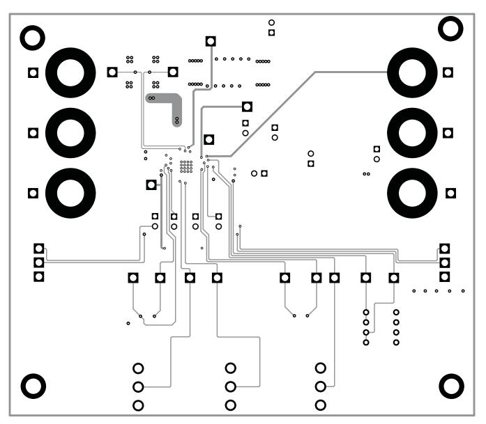
Figure 8. Layer 3 Routing
