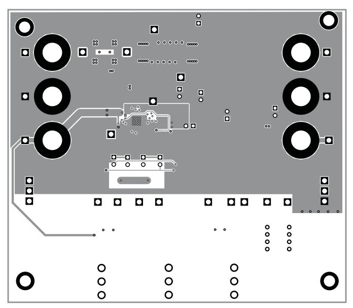
Figure 7. Layer 2 Routing
