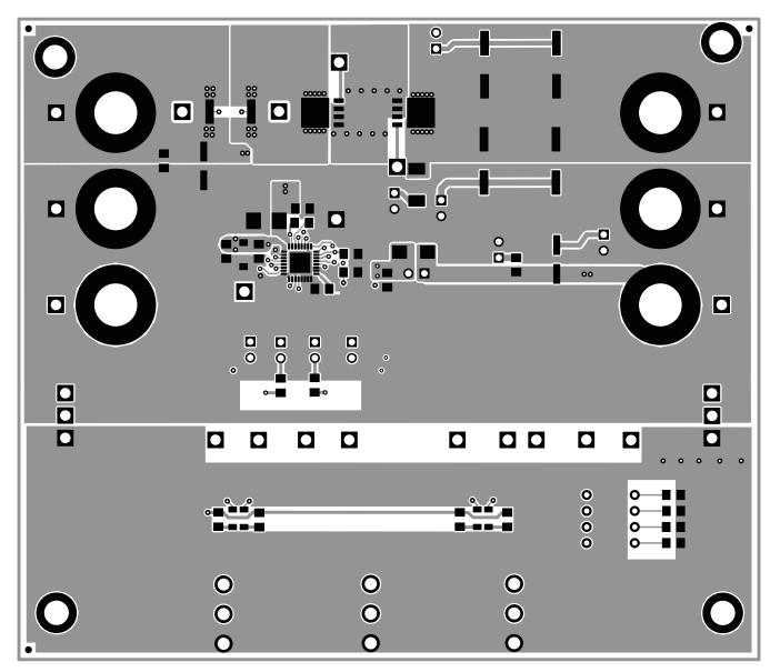
Figure 6. Top Layer Routing
