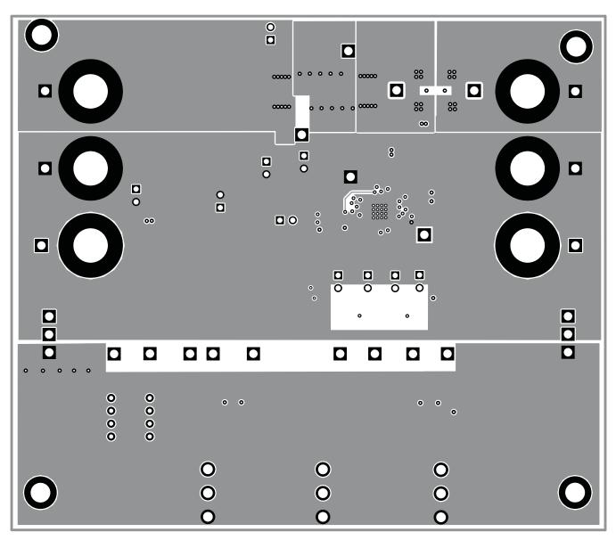
Figure 9. Bottom Layer Routing
