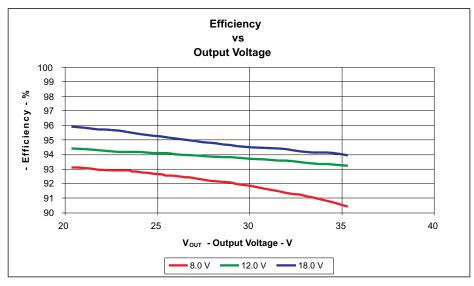
Figure 4. TPS40211EVM-352 Efficiency verse Output Voltage  $V_{IN}$  = 8 V to 18 V,  $I_{OUT}$  = 0.70 A,  $V_{OUT}$  = 20 V to 35 V
