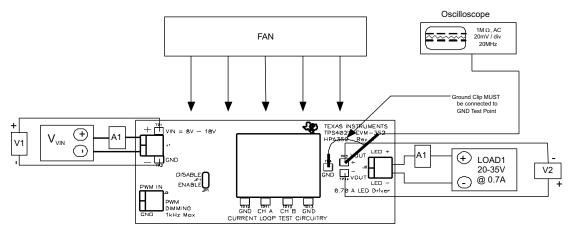
Figure 2. TPS40211EVM-352 Recommended Test Set-Up
