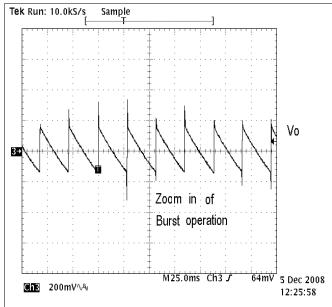
Figure 16. Typical Output Voltage in Burst Operation (TP15)
