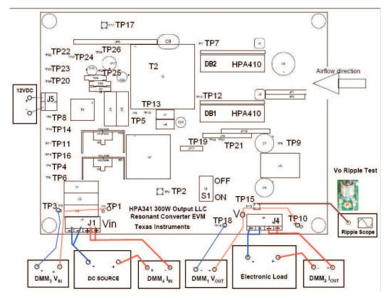
Figure 3. Recommended Test Set Up
