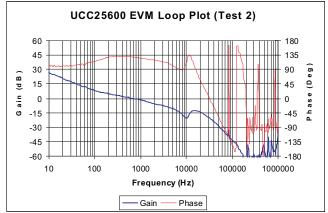
Figure 9. Full System Loop Compensation (TP19 and TP21)
