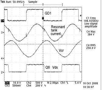
Figure 11. Typical Resonant Tank Current and Resonant Capacitor Voltage
