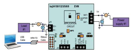
Figure 4. Test Setup for HPA255
