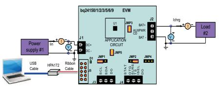
Figure 2. Original Test Setup for HPA255 (bq2415x EVM)
