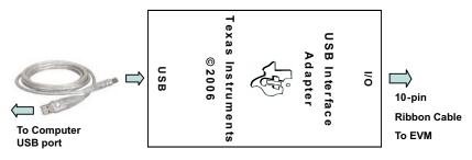
Figure 1. Connections of the HPA172 Kit
