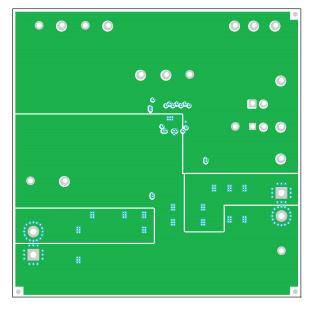
Figure 14. TPS40304EVM-353 Bottom Copper (Top view)
