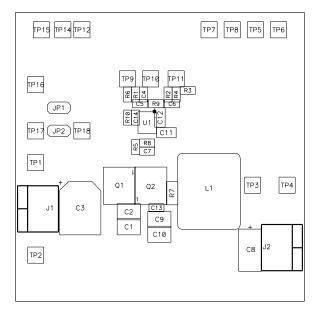
Figure 11. TPS40304EVM-353 Component Placement (Top view)
