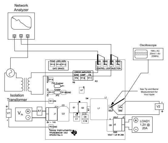
Figure 4. Control Loop Measurement Setup
