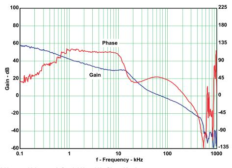
$V_{IN}$  = 14V,  $V_{OUT}$  = 1.2V,  $I_{OUT}$  = 20A, Bandwidth: 73kHz, Phase Margin: 47°
