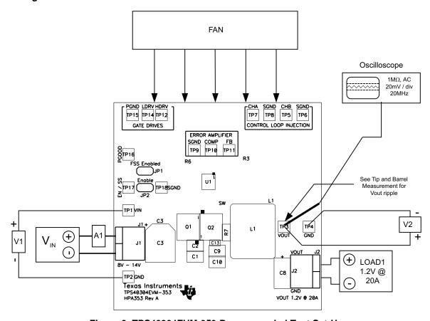
Figure 2. TPS40304EVM-353 Recommended Test Set-Up
