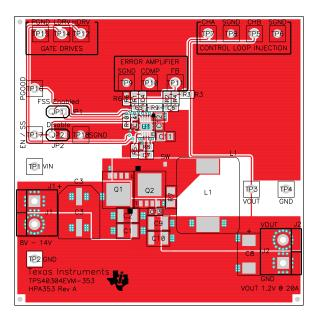
Figure 13. TPS40304EVM-353 Top Copper (Top view)
