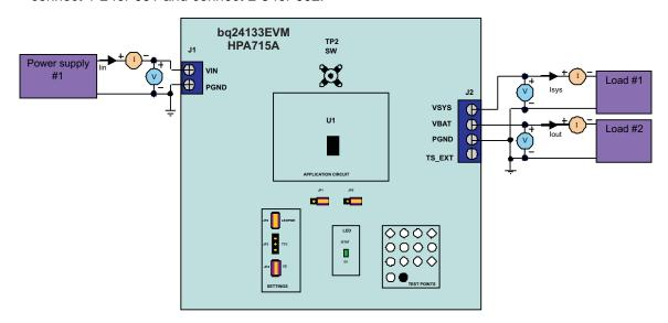
Figure 1. Original Test Setup for HPA715A (bq24133EVM)
