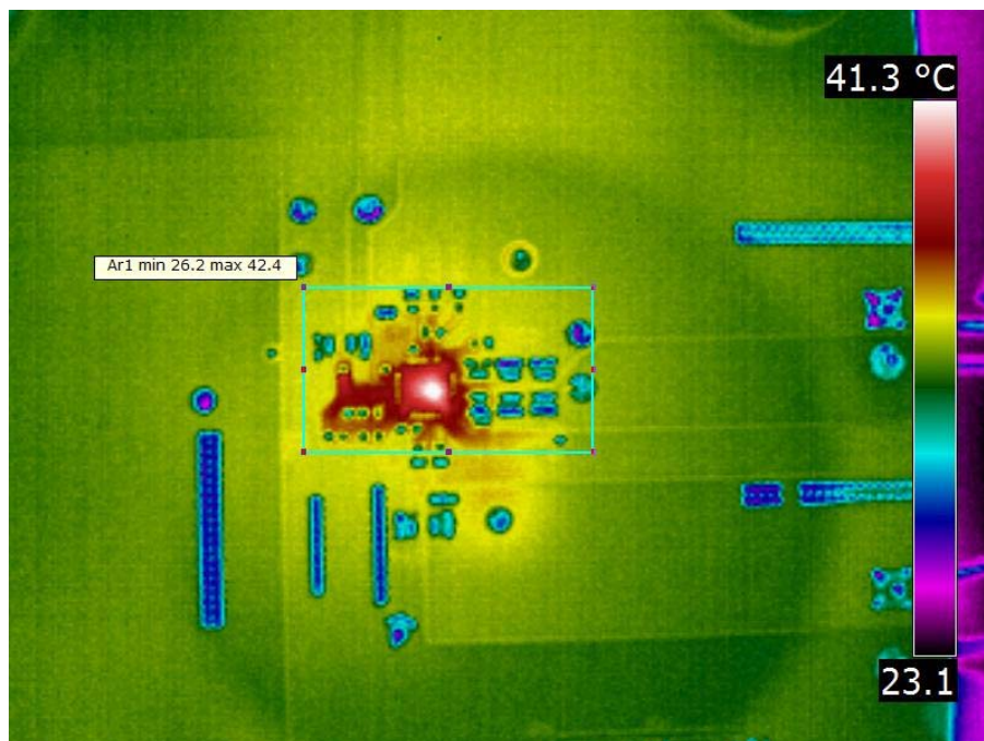
Back Side of EVM – Max Temp = 42.4°C
