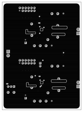
Figure 21. TPS53310EVM-755 Internal Layer 2, Top View
