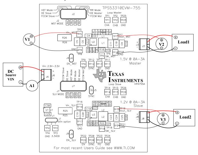
Figure 3. TPS53310EVM-755 Recommended Test Setup
