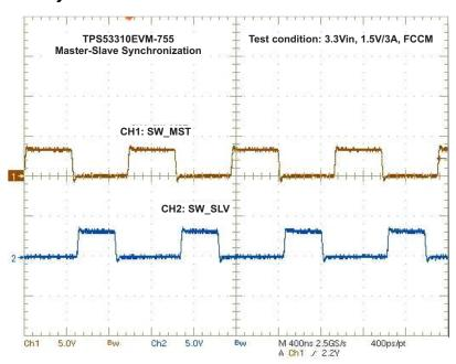
Figure 10. TPS53310EVM-755 Synchronization (3.3 Vin, 1.5 V/3 A, 1.2 V/3 A 180° Synchronization)
