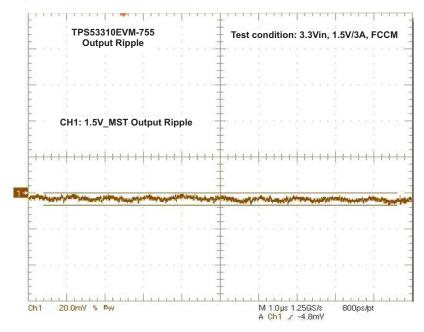
Figure 7. TPS53310EVM-755 Output Ripple (3.3 Vin, 1.5 V/3 A)
