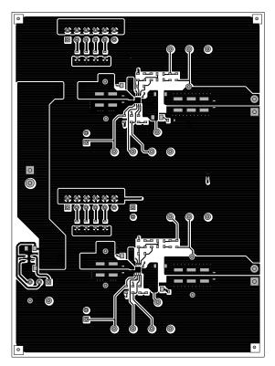
Figure 20. TPS53310EVM-755 Top Copper, Top View
