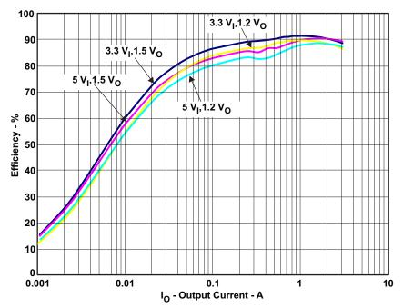
NOTE: R-C snubber to reduce switching node ringing has effect on dc-dc converter efficiency.
