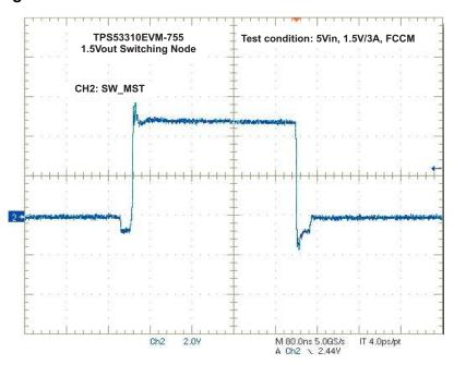
Figure 8. TPS53310EVM-755 Switching Node at Full Load (5 Vin, 1.5 V/3 A)
