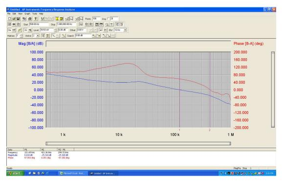
Figure 16. TPS53310EVM-755 Bode Plot (3.3 Vin, 1.5 V/3 A)
