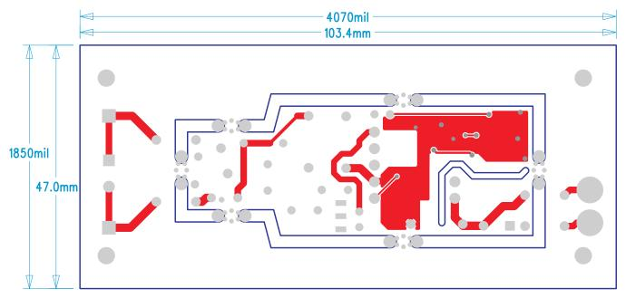
Figure 29. LM3447-A19-120VEVM Top Layer Copper (top view)
