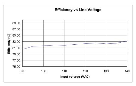
Figure 3. LM3447-A19-120VEVM Efficiency
