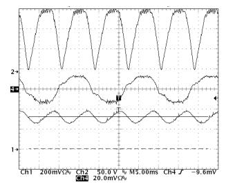
Figure 8. Output Ripple (Ch1 - LED current Ch2 - rectified line voltage Ch4- line current 200 mA/div)
