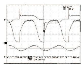
Figure 24. Pre-Short Circuit Waveforms (Ch4- LED current Ch2 - rectified line voltage Ch1 – line current)
