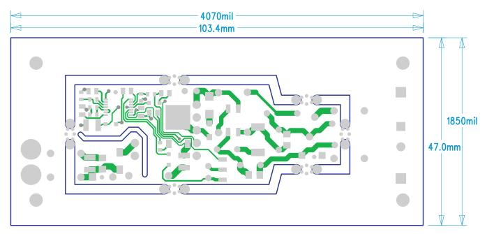
Figure 30. LM3447-A19-120VEVM Bottom Layer Copper (bottom view)
