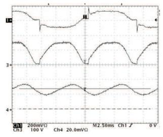
Figure 12. Dimmer Full (Ch4- LED current Ch3 - rectified line voltage Ch1 – line current)
