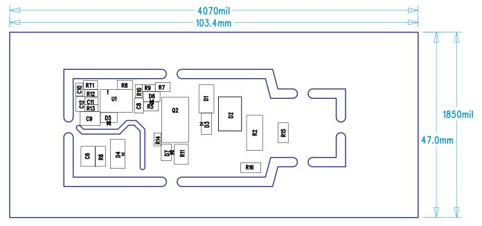
Figure 32. LM3447-A19-120VEVM Bottom Assembly Drawing (bottom view)
