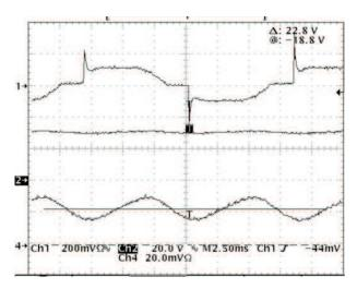
Figure 21. Pre-Open Circuit Waveforms (Ch4- LED current Ch2- LED voltage Ch1 – line current)
