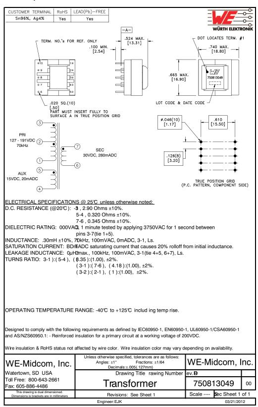
Figure 28. Transformer Specification
