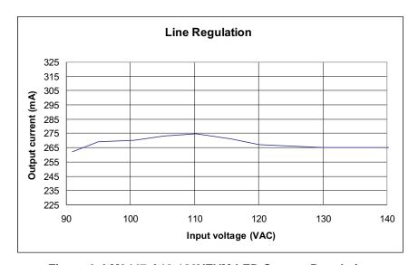
Figure 6. LM3447-A19-120VEVM LED Current Regulation
