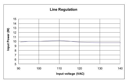
Figure 5. LM3447-A19-120VEVM Input Power Regulation
