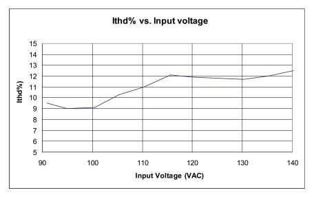
Figure 7. LM3447-A19-120VEVM- Ithd % vs Line Voltage
