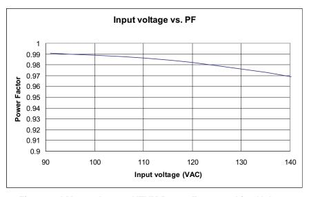
Figure 4. LM3447-A19-120VEVM Power Factor vs Line Voltage
