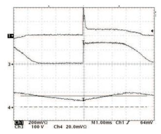
Figure 16. Dimmer 5 ms (Ch4- LED current Ch3 - rectified line voltage Ch1 – line current)
