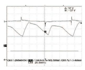
Figure 25. Short Circuit Waveforms (Ch4- LED current Ch2 - rectified line voltage Ch1 – line current)
