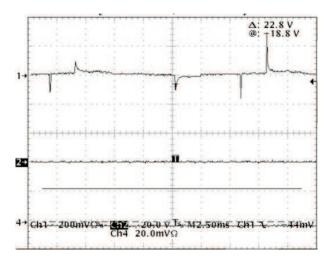
Figure 26. Short Circuit Waveforms (Ch4- LED current Ch2- LED voltage Ch1 – line current)
