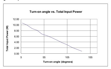
Figure 11. Turn-On Angle vs. Input Power
