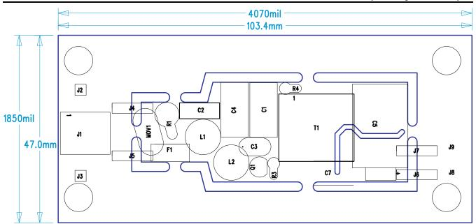
Figure 31. LM3447-A19-120VEVM Top Assembly Drawing (top view)
