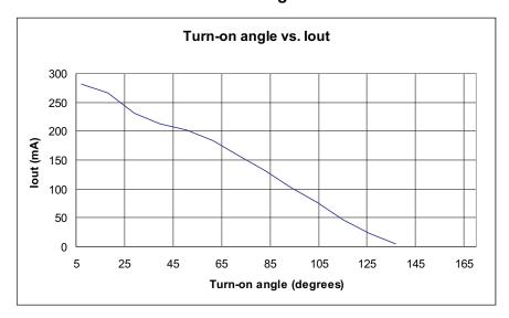
Figure 10. LED Current vs Conduction Angle
