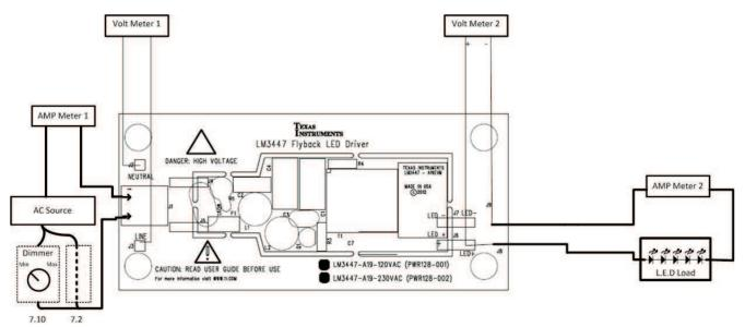
Figure 2. LM3447-A19-120VEVM Recommended Test Set Up
