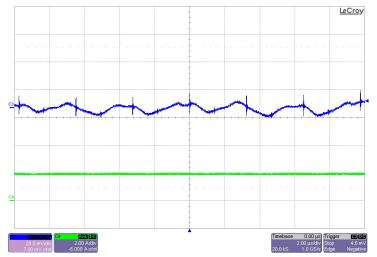
2.1A Load, Measured After the USB Switch at the End of an iPhone Cable
