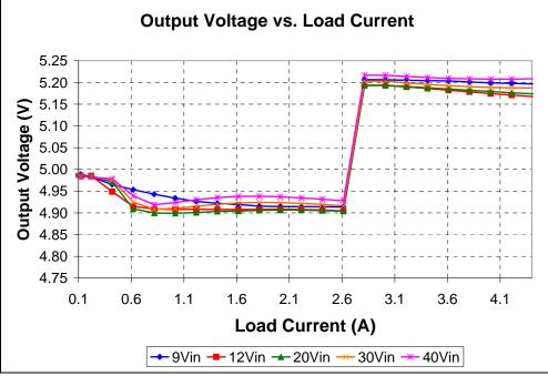
Output Load Regulation Before the USB Switch
