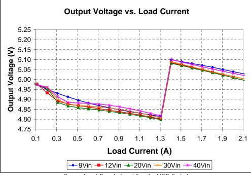
Output Load Regulation After the USB Switch
