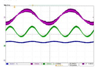
Figure 15. Pre-Open Circuit Waveforms (Ch1 - LED voltage (10V/div); Ch3 - line current (100mA/div); Ch4 - LED current(200mA/div))
