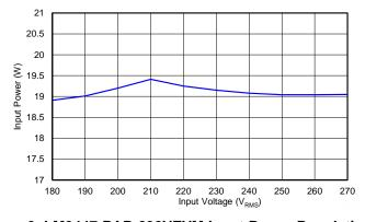
Figure 9. LM3447-PAR-230VEVM Input Power Regulation
