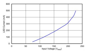
Figure 25. LED Current vs Input Voltage
