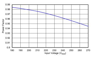
Figure 8. LM3447-PAR-230VEVM Power Factor vs Line Voltage
