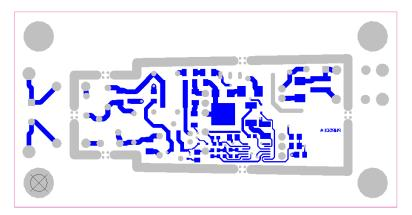
Figure 4. LM3447-PAR-230VEVM Bottom Layer Copper (bottom view)
