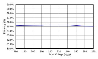
Figure 7. LM3447-PAR-230VEVM Efficiency
