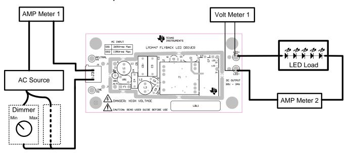
Figure 2. LM3447-PAR-230VEVM Recommended Test Set Up
