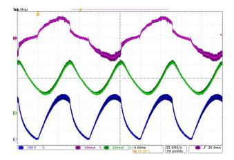
Figure 22. Dimmer at maximum brightness setting (Ch1 - rectified line voltage (100V/div); Ch3 - line current (100mA/div); Ch4- LED current (100 mA/div))
