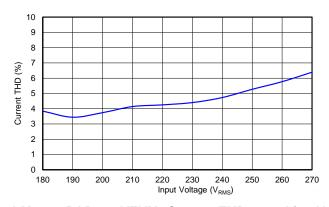
Figure 11. LM3447-PAR-230VEVM- Current THD % vs Line Voltage
