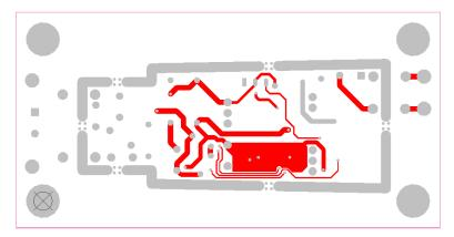
Figure 3. LM3447-PAR-230VEVM Top Layer Copper (top view)
