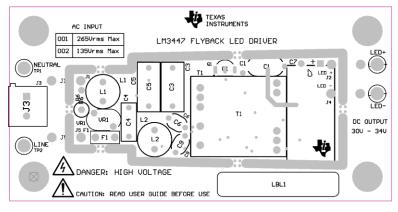
Figure 5. LM3447-PAR-230VEVM Top Assembly Drawing (top view)
