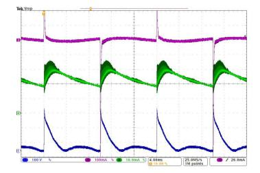
Figure 28. Dimmer at minimum brightness setting (Ch1 - rectified line voltage (100V/div); Ch3 - line current (100mA/div); Ch4- LED current (100 mA/div))
