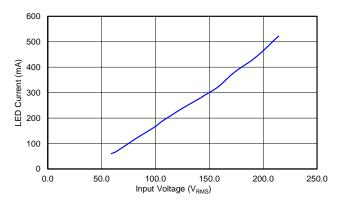
Figure 21. LED Current vs Conduction Angle
