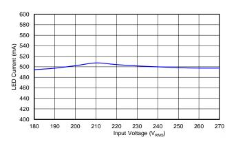
Figure 10. LM3447-PAR-230VEVM LED Current Regulation
