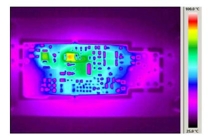
Figure 32. LM3447-PAR-230VEVM Thermal Image (bottom view)
