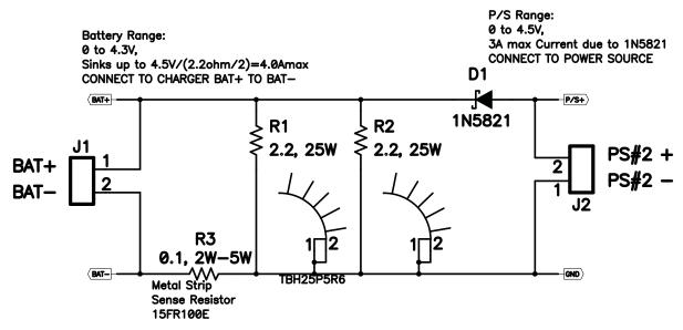
Figure 7. BAT Load (PR1010) Schematic
