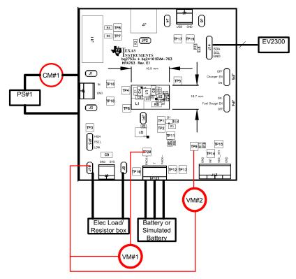
Figure 8. Original Test Setup for bq24160/161/163/168EVM (HPA721)
