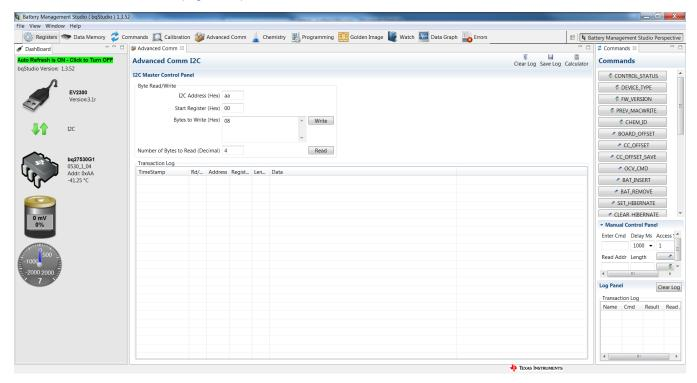
Figure 13. Advanced Communication I<sup>2</sup>C
