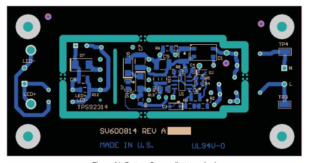
Figure 21. Bottom Copper (bottom view)
