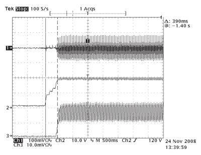
Figure 13. Enable Turn-On Delay (Ch1 - Input Current Ch2 - LED Voltage Ch3 - LED Current (200 mA/div))
