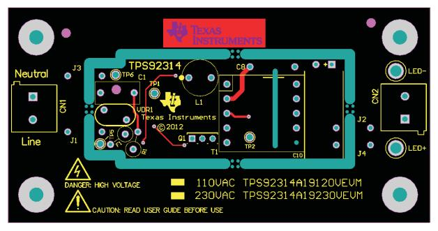
Figure 20. Top Copper (top view)
