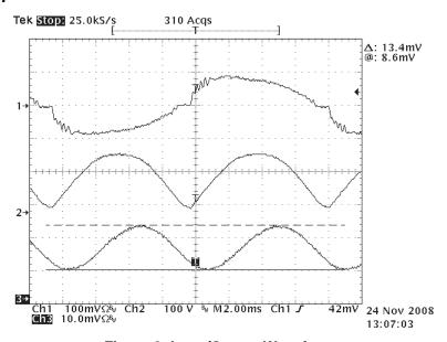
Figure 9. Input/Output Waveforms (Ch1 - Input current Ch2 - Rectified Line Voltage Ch3 - LED Current (200 mA/div))
