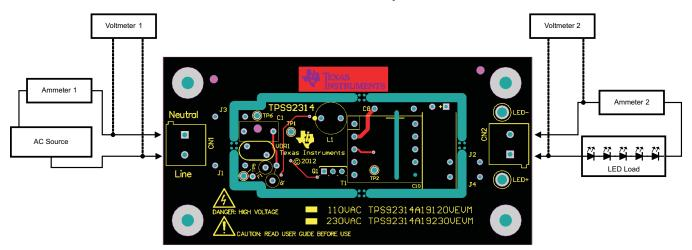
Figure 2. Recommended Test Set Up
