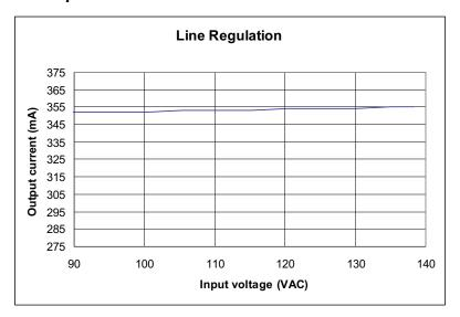
Figure 5. Current Variation with Respect to Input Voltage
