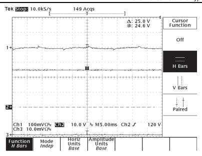
Figure 15. LED Open Circuit Waveforms (Ch1 - Input current Ch2 - LED Voltage Ch3 - LED Current (200 mA/div))
