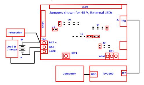
Figure 8. bq34z110 Circuit Module Connection to Cells and System Load and Charger
