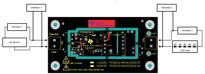
Figure 2. Recommended Test Setup
