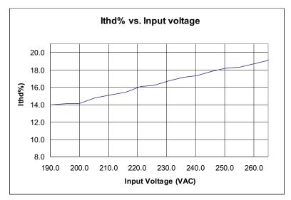
Figure 7. Ithd% vs Input Voltage
