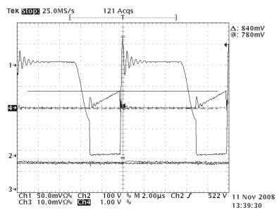
Figure 11. Current Sense Waveform (Ch2 - Switch Node Voltage, Ch3 - LED Current (200 mA/div), Ch4 - Current Sense Voltage)
