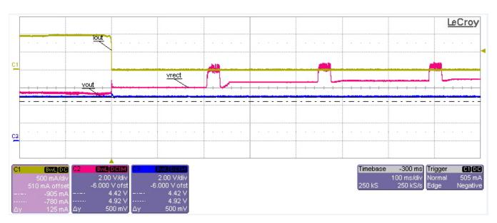
Figure 4. Load Dump, 500 mA to 0 mA
