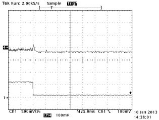
Figure 9. 0.1-A to 0.6-A Load Step
