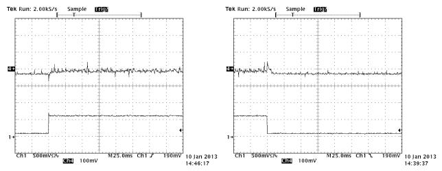
Figure 10. 0.6-A to 0.1-A Load Step
