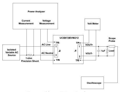
Figure 2. UCC28720EVM-212 Test Setup
