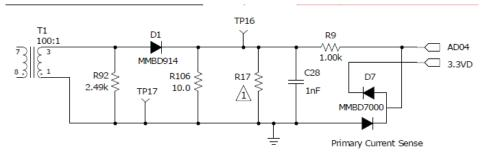
Figure 45. Cycle-by-Cycle Current Limit Sensing Circuit
