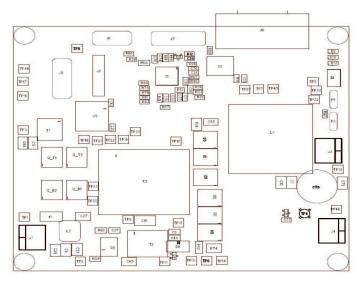
Figure 15. UCD3138HSFBEVM-029 Top Layer Assembly Drawing (top view)
