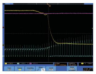
Figure 48. Short Circuit Protection Test
