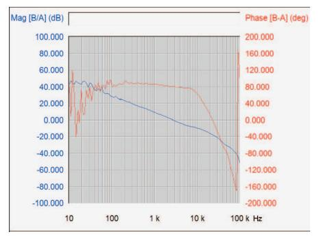
Figure 14. Control Loop Bode Plots at 48  $V_{\mbox{\tiny DC}}$  and Full Load
