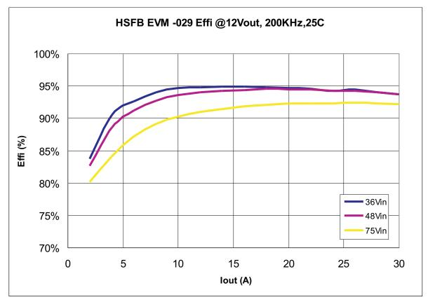
Figure 6. UCD3138HSFBEVM-029 Efficiency
