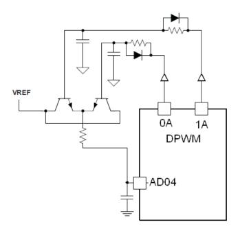
Figure 46. An Example of External Slope Compensation
