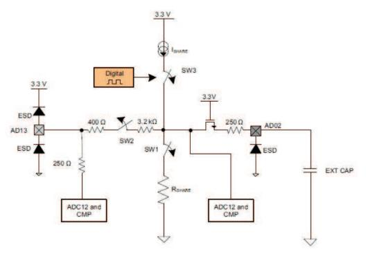
Figure 28. UCD3138 Load Sharing Module
