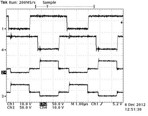
Figure 32. Normal Operation Switching Waveforms
