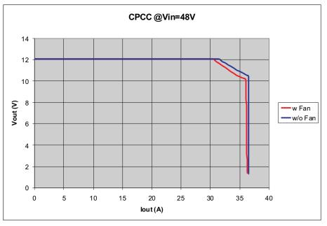
Figure 43. Constant Power Constatnt Current Operation
