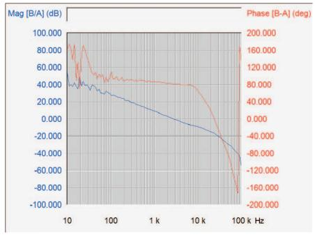
Figure 13. Control Loop Bode Plots at 48  $V_{\mbox{\tiny DC}}$  and Half Load
