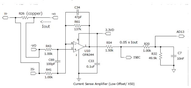
Figure 27. Load Current Sensing by PCB Copper
