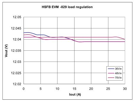
Figure 7. UCD3138HSFBEVM-029 Load Regulation
