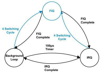
Figure 30. Firmware Structure Overview
