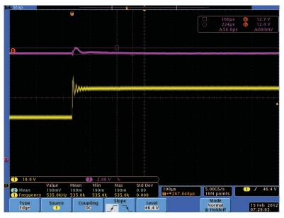
Figure 39. V<sub>o</sub> Change from Digital Feed Forward Control
