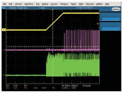
Figure 11. Output Turn On 48  $V_{DC}$  with Load Range (Ch 1 =  $V_0$ , Ch 3 = DPWM1B, Ch 4 =  $V_{CT}$ , Load = 1 A)
