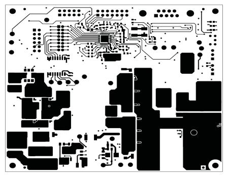
Figure 17. UCD3138HSFBEVM-029 Top Copper (top view)
