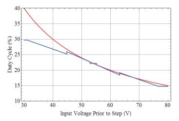
Figure 37. Duty Cycle Change in Feed Forward Control
