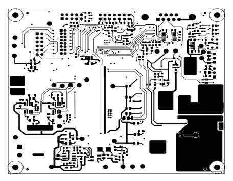
Figure 20. UCD3138HSFBEVM-029 Bottom Copper (top view)
