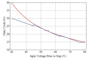
Figure 38. UCD3138 Digital Feed-Forward Control
