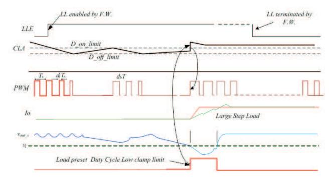
Figure 41. Burst Operation Timing Diagram
