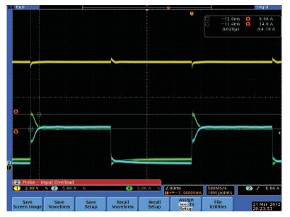
Figure 36. Current Sharing Test
