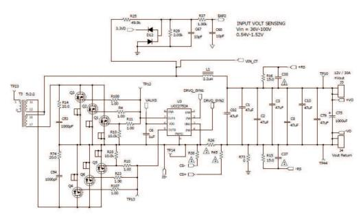
Figure 26. Input Voltage Sensing Using Main Transformer
