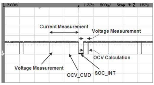
Figure A-2. OCV Calculation Based on OCV Command
