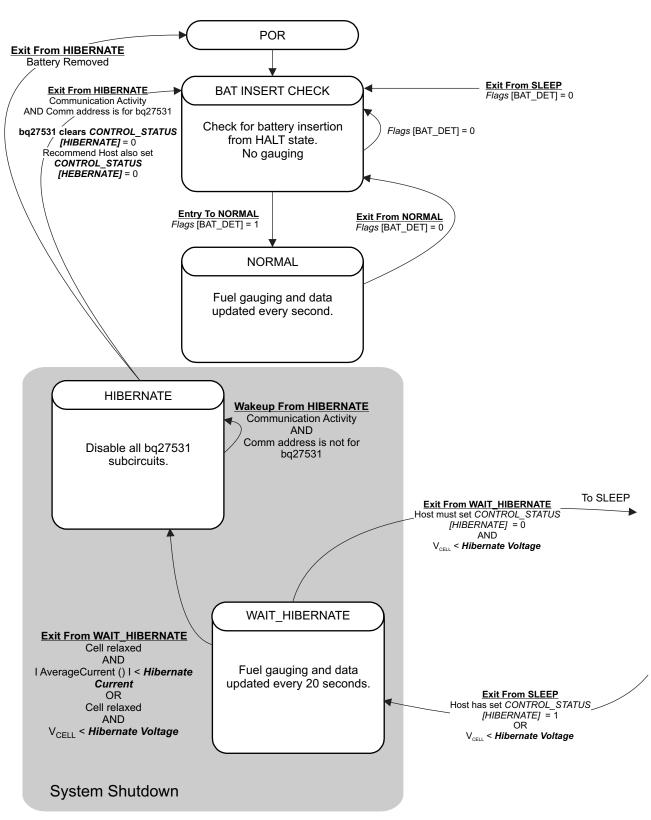
Figure 6-2. Power Mode Diagram—System Shutdown
