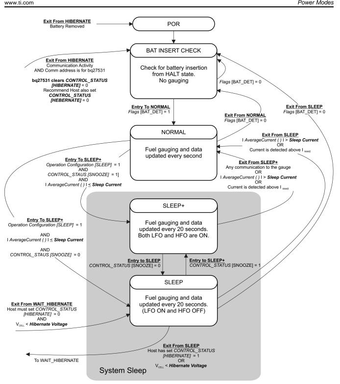
Figure 6-1. Power Mode Diagram—System Sleep
