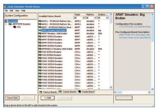
Figure 13. Setup Code Composer Studio v3.3 for UCD3138
