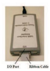
Figure 3. USB-to-GPIO Interface Adapter Outlook
