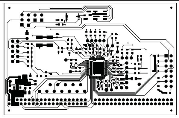
Figure 9. UCD3138064EVM-166 Top Copper (top view)
