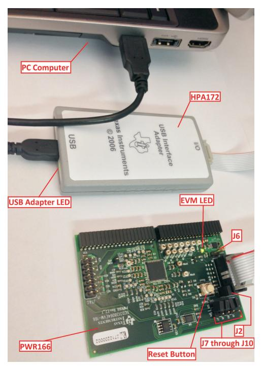
Figure 4. UCD3138064EVM-166 Test Connections
