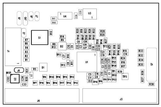
Figure 7. UCD3138064EVM-166 Top Layer Assembly Drawing (top view)
