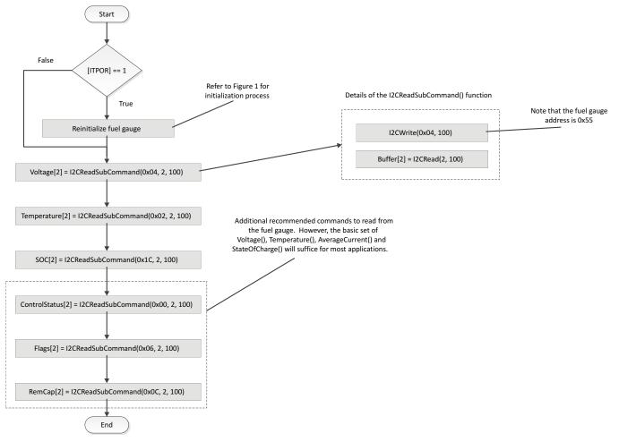
Figure 2. Gauge Register Commands
