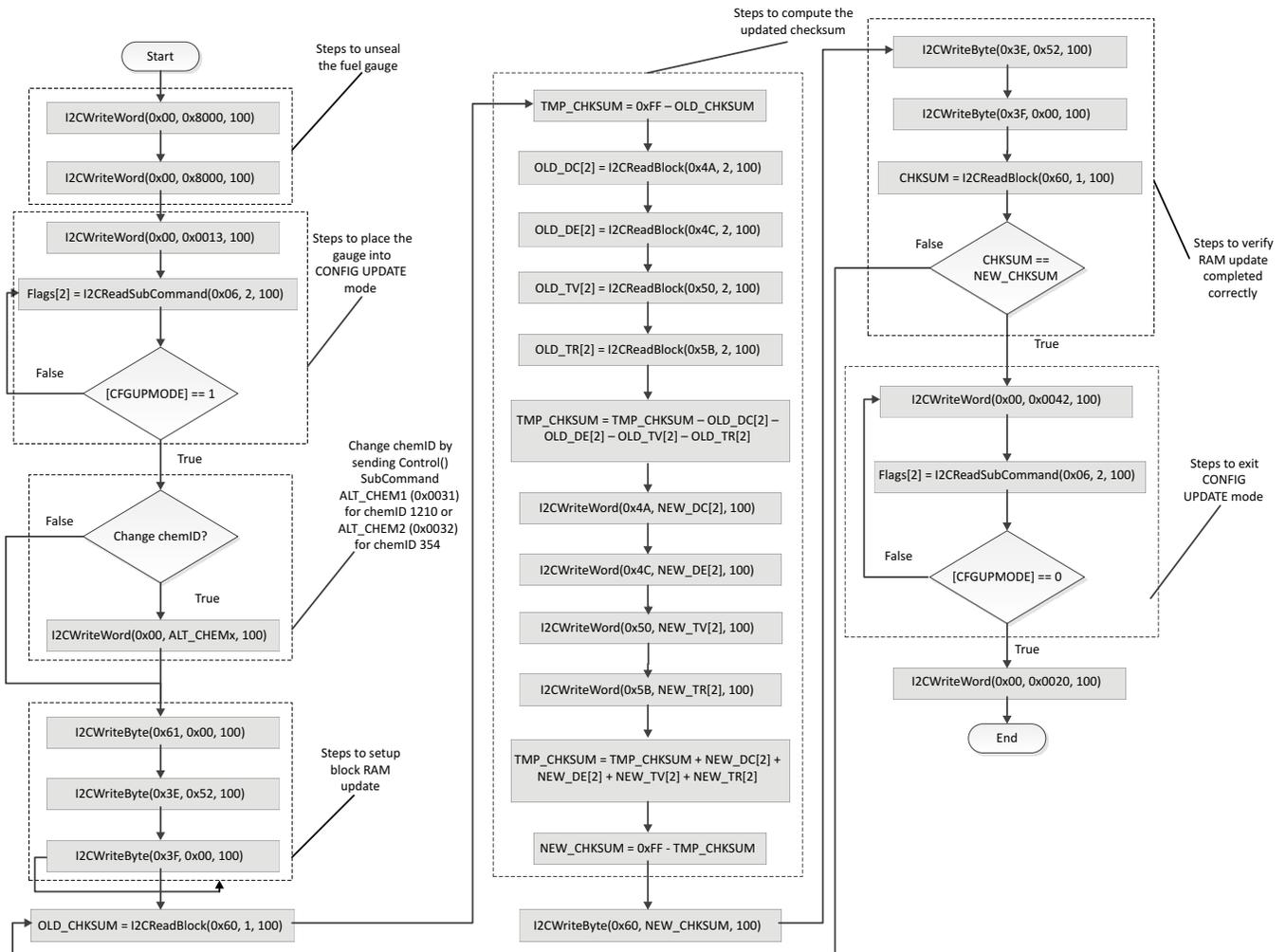
**Figure 1. Flowchart for Updating the Gauge Configuration Parameters**
