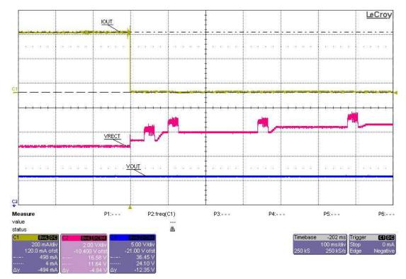
Figure 4. Load Dump, 500 mA to 0 mA
