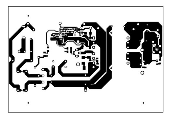
Figure 20. UCC28630EVM-572 Bottom Copper (bottom view)
