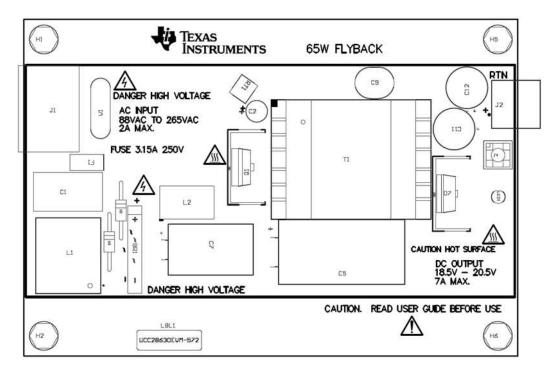
Figure 17. UCC28630EVM-572 Top Layer Assembly Drawing (top view)
