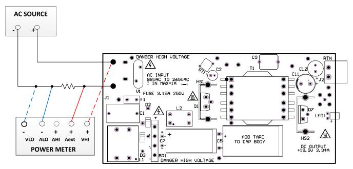
Figure 2. Test Setup
