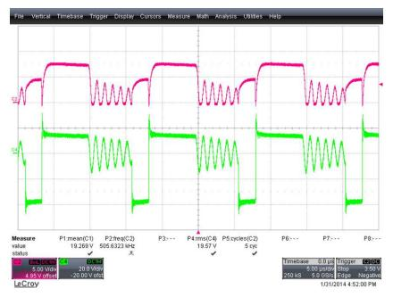
Figure 13. Bias Winding and VSENSE Pin Voltage Waveforms
