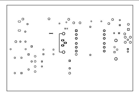
Figure 19. UCC28630EVM-572 Top Copper (top view)
