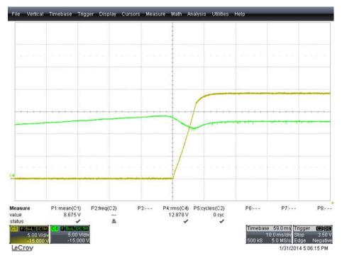
Figure 12. Output Voltage Turn-On Waveform
