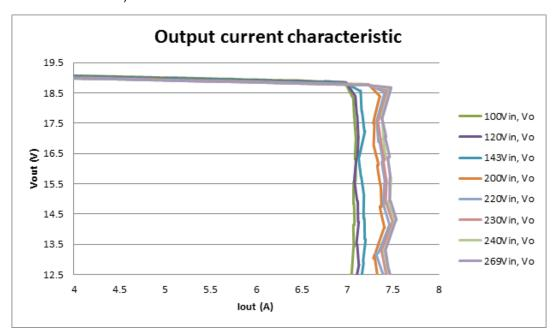
Figure 7. UCC28630EVM-572 Output Voltage as a Function of Load Current
