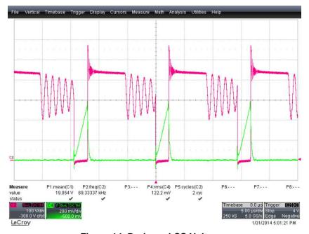
Figure 14. Drain and CS Voltages
