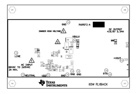
Figure 18. UCC28630EVM-572 Bottom Layer Assembly Drawing (bottom view)
