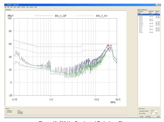
Figure 16. 230-V<sub>AC</sub> Conducted Emissions Plot
