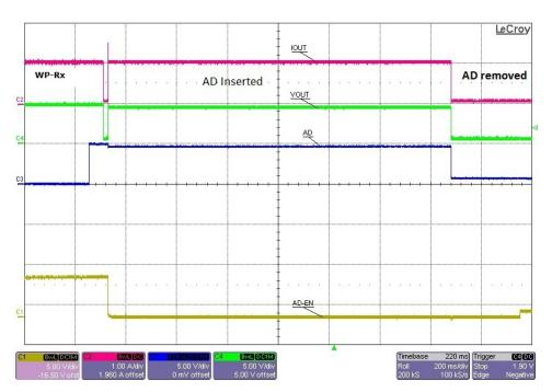
Figure 6. Adapter Insertion and Removal
