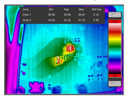
Figure 7. Thermal Image (1000-mA Load)
