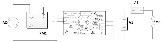
Figure 2. UCC28880EVM-615 Test Set Up
