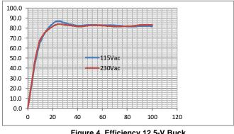
Figure 4. Efficiency 12.5-V Buck
