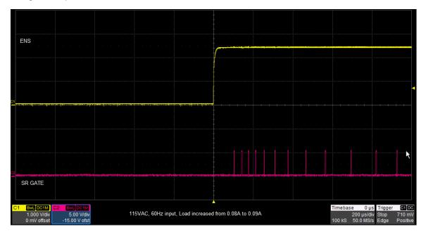
Figure 18. ENS and SR GATE as Load Increases
