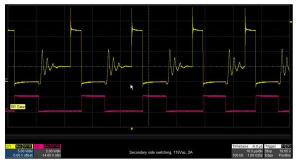
Figure 15. Secondary Side Switching Waveform
