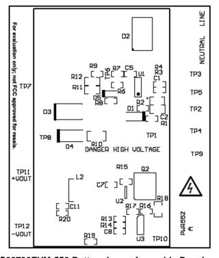
Figure 20. UCC28730EVM-552 Bottom Layer Assembly Drawing (Bottom view)
