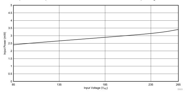
Figure 6. UCC28730EVM-552 No-Load Power Consumption
