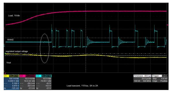
Figure 9. UCC28730EVM-552 WAKE Signal During Load Transient
