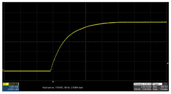
Figure 12. Output Voltage Turn On Waveform
