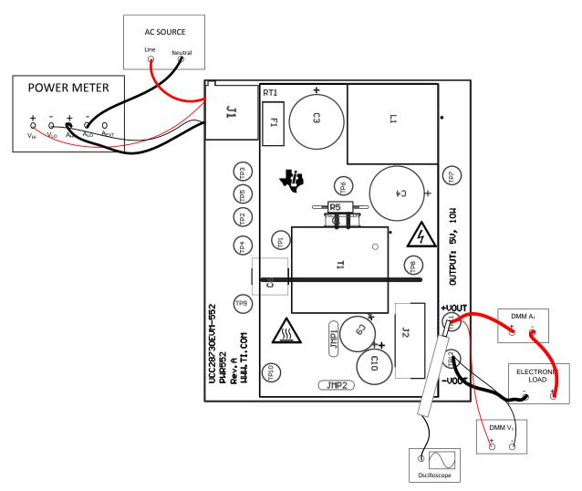
Figure 3. FUCC28730EVM-552 Recommended Test Set Up With Load
