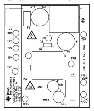
Figure 19. UCC28730EVM-552 Top Layer Assembly Drawing (Top view)
