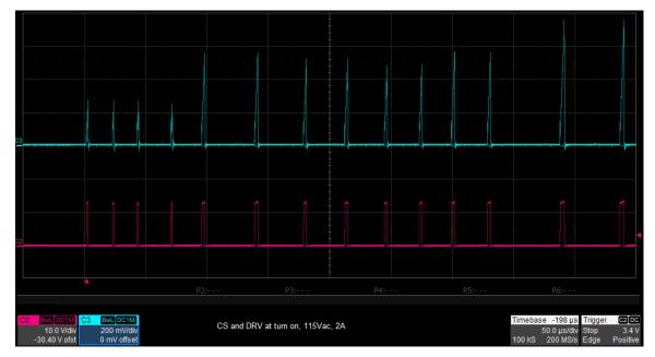
Figure 13. CS and DRV at Turn On
