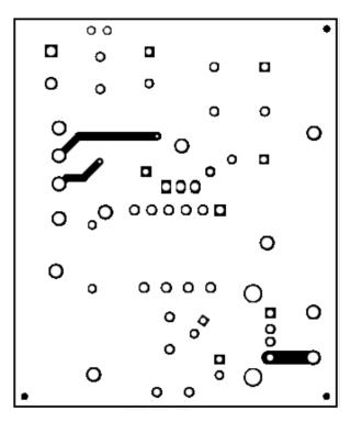
Figure 21. UCC28730EVM-552 Top Copper (Top View)
