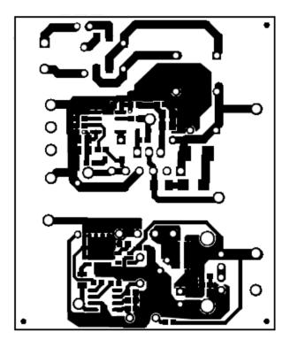
Figure 22. UCC28730EVM-552 Bottom Copper (Bottom View)
