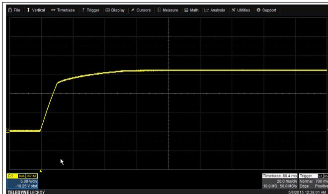
Figure 4.  $V_{IN} = 85 V_{RMS}$ ,  $I_{OUT} = 0 A$
