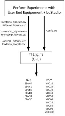
Figure 5. CEDV Coefficients Calculation Flow
