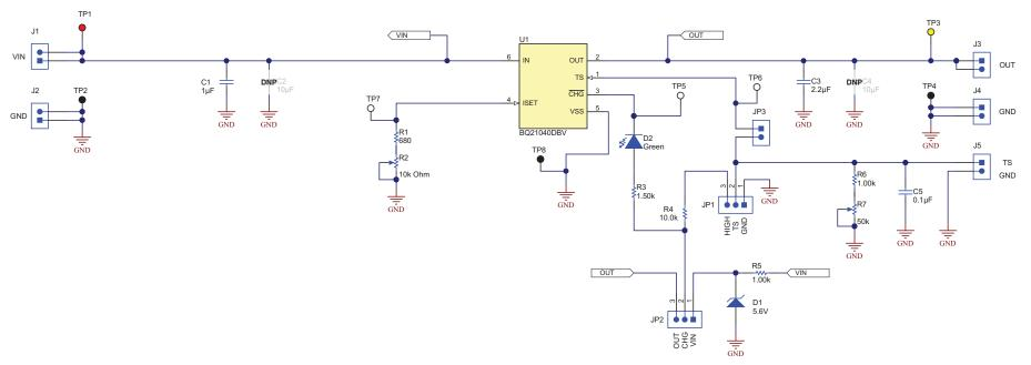
Figure 2. bq21040 EVM Board Schematic
