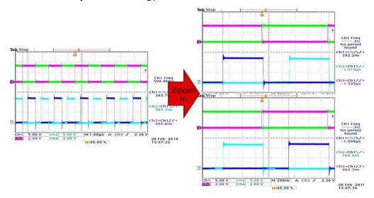
Figure 7-3. Test Waveforms if DT Connected to R<sub>DT</sub> (Channel 3 and 4 is PWM Inputs, and Channel 1 and 2 is Driver Outputs)
