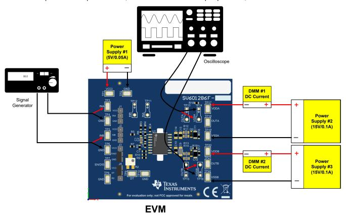
Figure 5-2. Bench Setup Diagram and Configuration
