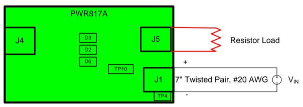
Figure 2. Typical TPS254900Q1EVM-817 Test Setup
