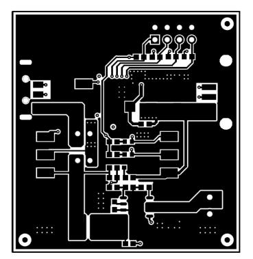
Figure 4. Top Side Routing
