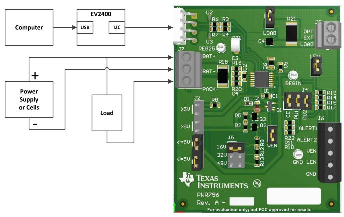
Figure 1. bq34110 Circuit Module Connection to Pack and System Load
