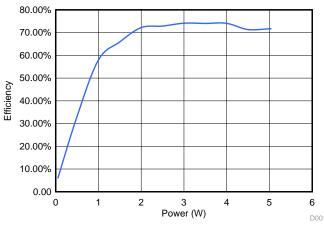
Figure 2. Efficiency vs Power, bq50002AEVM-607 TX and bq51013BEVM-764 Receiver
