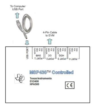
Figure 5. Connections of the EV2400 kit
