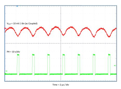
Figure 8. TPS54308EVM-876 Output Ripple,  $I_{OUT} = 10 \text{ mA}$
