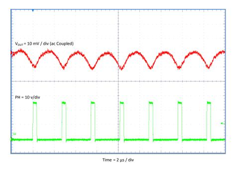
Figure 9. TPS54308EVM-876 Output Ripple,  $I_{OUT} = 0$  A
