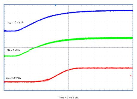
Figure 11. TPS54308EVM-876 Startup Relative to VIN
