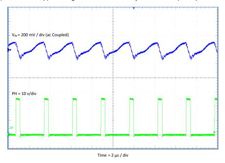
Figure 10. TPS54308EVM-876 Input Ripple
