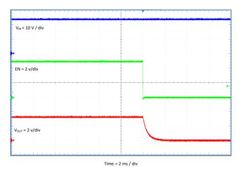
Figure 14. TPS54308EVM-876 Shutdown Relative to EN
