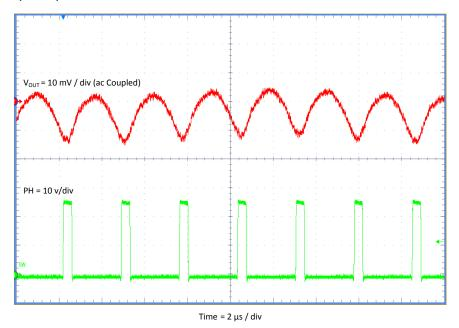
Figure 6. TPS54308EVM-876 Output Ripple, I<sub>OUT</sub> = 3 A
