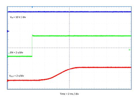
Figure 12. TPS54308EVM-876 Startup Relative to Enable
