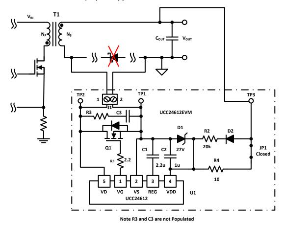
Figure 4. UCC24612-1EVM Used in Low-Side Rectifier Application
