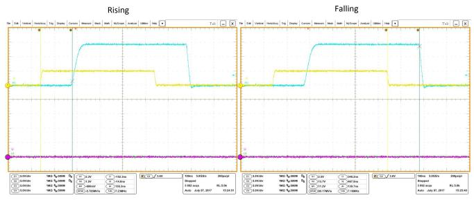
Figure 3. HI and HO Waveforms if Input Dead Time is Greater Than Internal Dead Time (Yellow and Magenta are PWM Inputs, Green and Blue are Driver Outputs)
