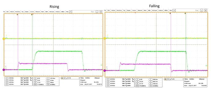
Figure 4. LI and LO Waveforms if Input Dead Time is Greater Than Internal Dead Time (Yellow and Magenta are PWM Inputs, Green and Blue are Driver Outputs)
