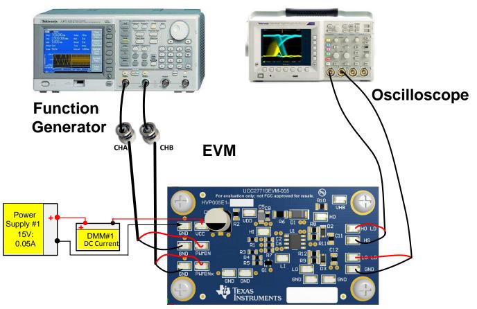
Figure 1. Bench Setup Diagram and Configuration
