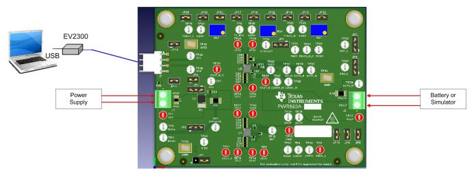
Figure 1. Test Setup for BQ25970
