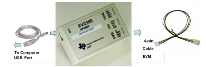
Figure 2. Connections of the EV2300 Kit
