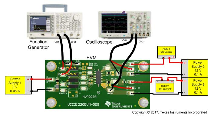
Figure 2. Bench Setup Diagram and Configuration
