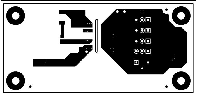
Figure 8. Bottom Layer (Flipped)
