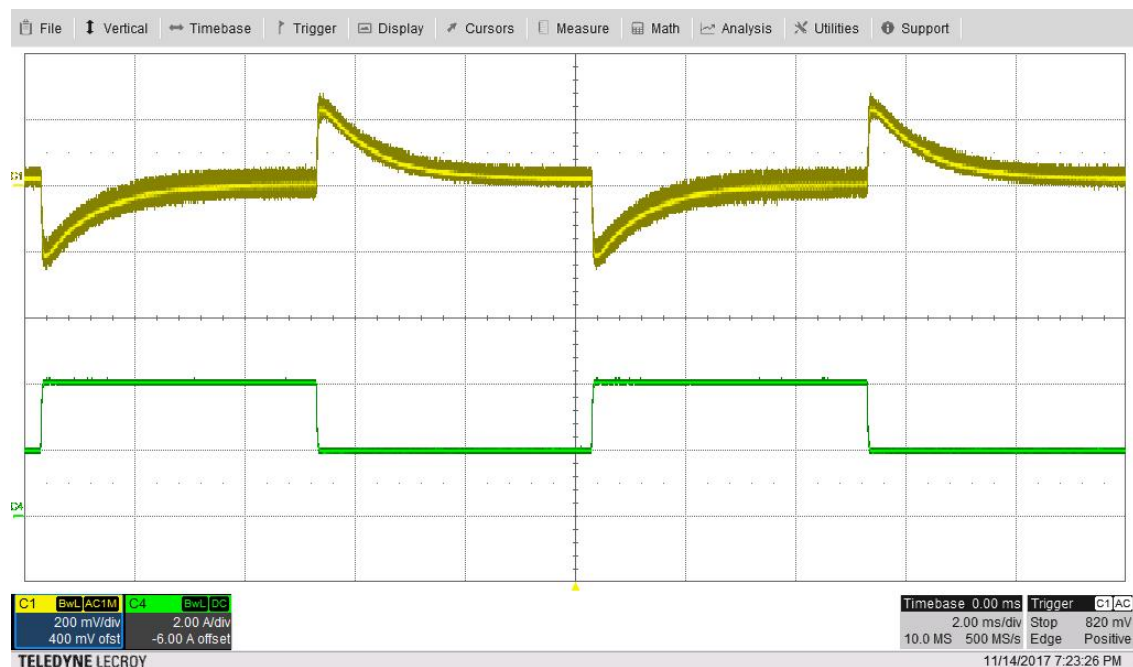
Figure 5. Transient Response from 2 A to 4 A for a 48-V Input
