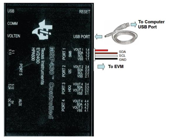
The picture shows the SMBus version EVM connection. If using the BQ25713EVM-017, move the connector to the  $I^{2}C$  port.
