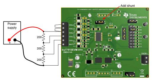
Figure 3. Operation With Reduced Cell Count
