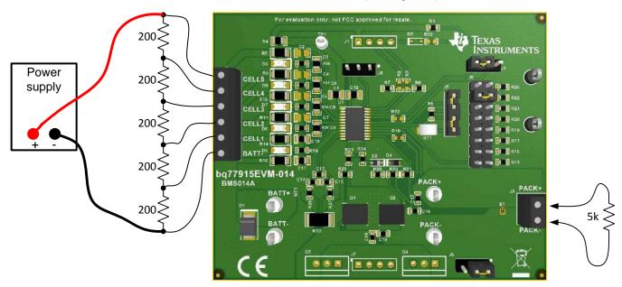
Figure 1. bq77915 Circuit Module Connection for Simple Demonstration
