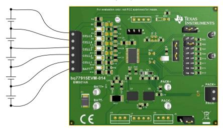
Figure 4. Connecting to Cells
