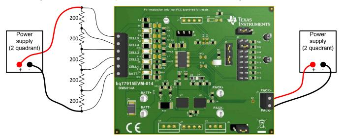
Figure 2. Bipolar Operation
