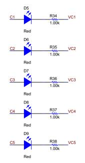
Figure 13. bq77915EVM Cell Balance Indicator Schematic
