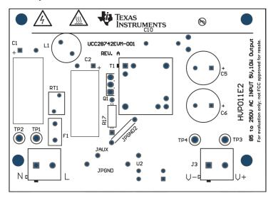
Figure 24. EVM Assembly (Top View)
