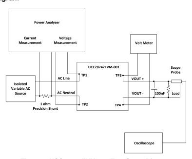
Figure 3. UCC28742EVM-001 Test Setup Diagram
