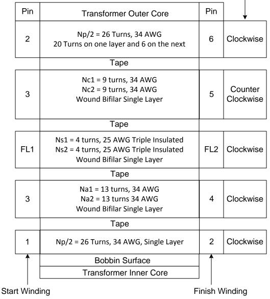
Figure 23. Transformer Winding Structure
