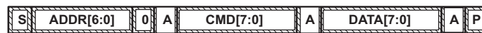
Figure 4-2. Attempt To Write a Read-Only Address (Nack After Data Sent By Master)
