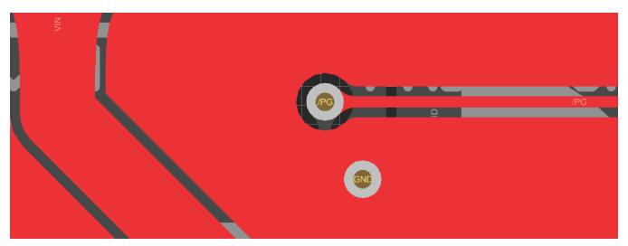
Figure 4. 40-mil VIN Trace (Left) Significantly Larger Than 6 mil / PG Trace (Center Right) for Current Capacity
