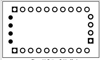
Figure 14. Bottom Solder Mask
