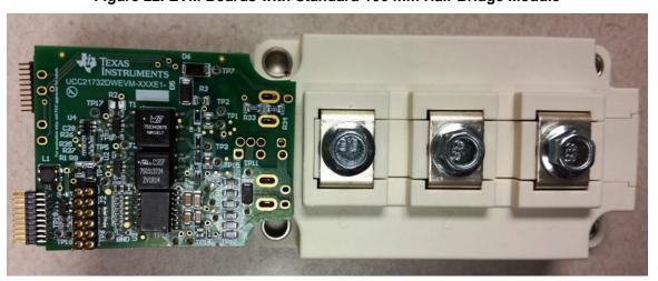
In 106-mm half-bridge module configuration two boards are placed one on top of another and the bottom board is flipped over. The supply voltage and input signals are provided through connectors J1 on each board. By connecting IN+ and INE- terminals on one board to INE+ and IN- terminals accordingly on another board, the overlapping protection circuit using logic U5 is engaged. This circuit could be disabled by removing resistors R31 and R32 in case of overlapping is required in the system.
