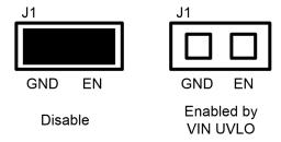
Figure 2-1. Enable Jumper Setting
