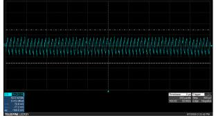
Figure 8-23. Typical Ripple Voltage of V<sub>OUT</sub> = 20 V
