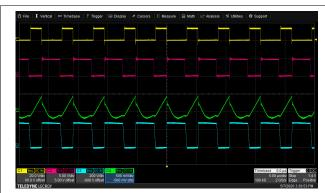
Figure 8-9. Typcial Waveform in AAM Operation Yellow = PWML, Red = PWMH, Green = Transformer Primary Winding Current (0.2 V/A), Blue = Switch Node Voltage
