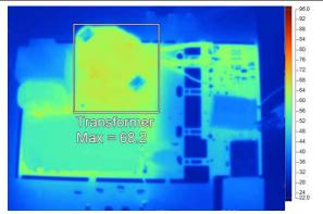
Figure 8-42.  $V_{IN}$  = 115  $V_{AC}$ , Top Side
