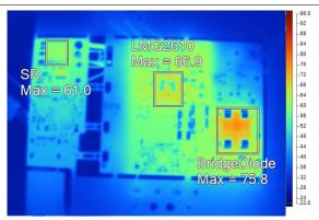
Figure 8-43.  $V_{IN}$  = 115  $V_{AC}$ , Bottom Side
