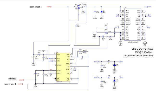
Figure 5-2. UCC28782EVM-030 Schematic Diagram (2 of 2)
