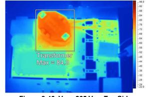
Figure 8-46.  $V_{IN}$  = 265  $V_{AC}$ , Top Side
