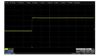
Figure 8-19. 5-V Output Power On
