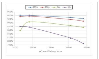
Figure 8-3. Full-load Efficiency vs. Input Voltage
