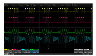
Figure 8-10. Typical Waveform in ABM Operation Yellow = PWML, Red = PWMH, Green = Transformer Primary Winding Current (0.2 V/A), Blue = Switch Node Voltage
