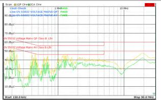
Figure 8-39. VIN = 230 V<sub>RMS</sub>, VOUT = 20 V, Load = 3.25 A (Output Not Grounded to LISN Ground, Ref Fig 54 and 55)
