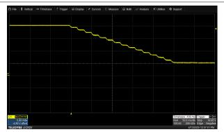
Figure 8-17. USB-C PD Output Change from 5 V to | Figure 8-18. USB-C PD Output Change from 20 V to 5 V
