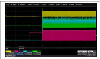
Figure 8-16. 230 V<sub>AC</sub> and Full Load Startup
