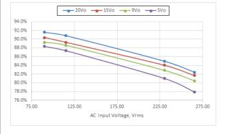
Figure 8-1. 4pt-Average Efficiency vs. Input Voltage
