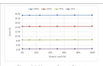
Figure 8-5. V<sub>OUT</sub> at Full-Load vs. Input Voltge
