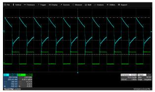
Figure 8-35. Transient Response at V<sub>OUT</sub> = 15 V Overshoot / Undershoot = 366 mV / -562 mV
