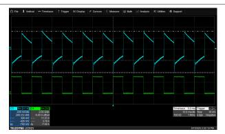
Figure 8-37. Transient Response at V<sub>OUT</sub> = 5 V Overshoot / Undershoot = 326 mV / -426 mV
