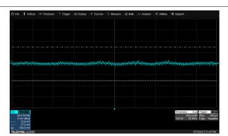
Figure 8-27. Typical Ripple Voltage of  $V_{OUT}$  = 5 V at | Figure 8-28. Typical Ripple Voltage of  $V_{OUT}$  = 5 V at **Full Load**
