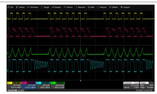
Figure 8-11. Typical Waveform in ABM Operation Yellow = PWML, Red = Vgs of SR MOSFET, Green = Transformer Primary Winding Current (0.2 V/A), Blue = Switch Node Voltage
