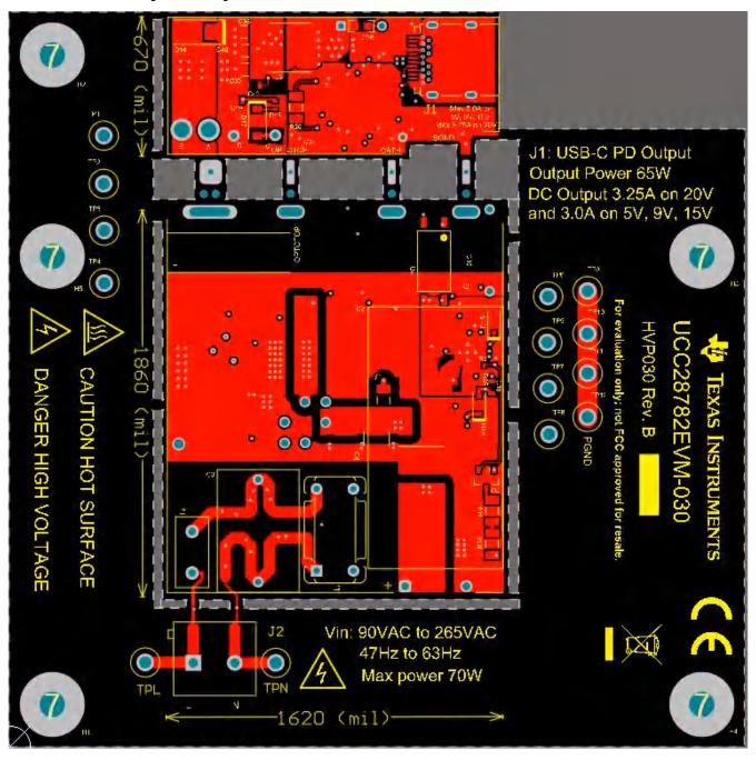
Figure 10-1. EVM Assembly (Top View)
