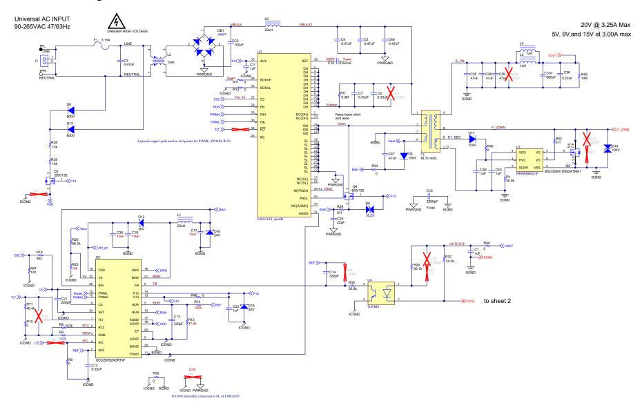
Figure 5-1. UCC28782EVM-030 Schematic Diagram (1 of 2), Updated October 2022 with LMG2610 integrated GaN half-bridge.
