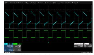
Figure 8-36. Transient Response at V<sub>OUT</sub> = 9 V Overshoot / Undershoot = 326 mV / -426 mV
