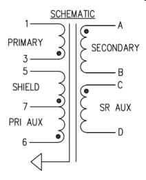
Figure 9-1. Transformer Schematic Diagram
