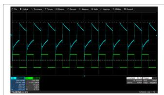
Figure 8-34. Load Transient Response at V<sub>OUT</sub> = 20 V Overshoot / Undershoot = 357 mV / -619 mV
