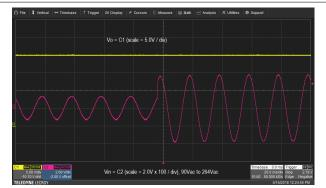
Figure 8-22. Output Voltage Response to Line Transient with No Load.
