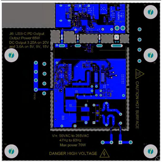
Figure 10-2. EVM Assembly (Bottom View)
