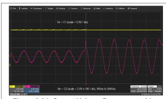
Figure 8-21. Output Voltage Response to Line Transient with Full Load.
