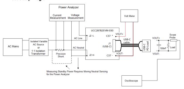
Figure 7-1. UCC28782EVM-030 Test Setup Diagram
