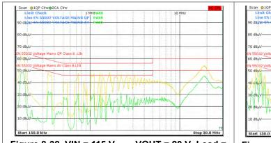
Figure 8-38. VIN = 115  $V_{RMS}$ , VOUT = 20 V, Load = 3.25 A (Output Not Grounded to LISN Ground, Ref Fig 54 and 55)
