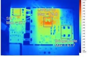
Figure 8-47.  $V_{IN}$  = 265  $V_{AC}$ , Bottom Side
