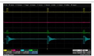
Figure 8-14. Typical Waveform in SBP2 Operation Yellow = PWML, Red = PWMH, Green = Transformer Primary Winding Current (0.2 V/A), Blue = Switch Node Voltage
