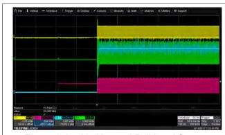
Figure 8-15. 115 V<sub>AC</sub> and Full Load Startup
