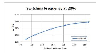
Figure 8-7. Average Switching Frequency vs. Input at 20-Vo Full Load
