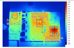
Figure 8-41.  $V_{IN}$  = 90  $V_{AC}$ , Bottom Side
