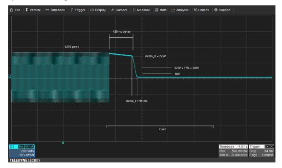
Figure 8-31. Typical X-Capacitor Discharge
