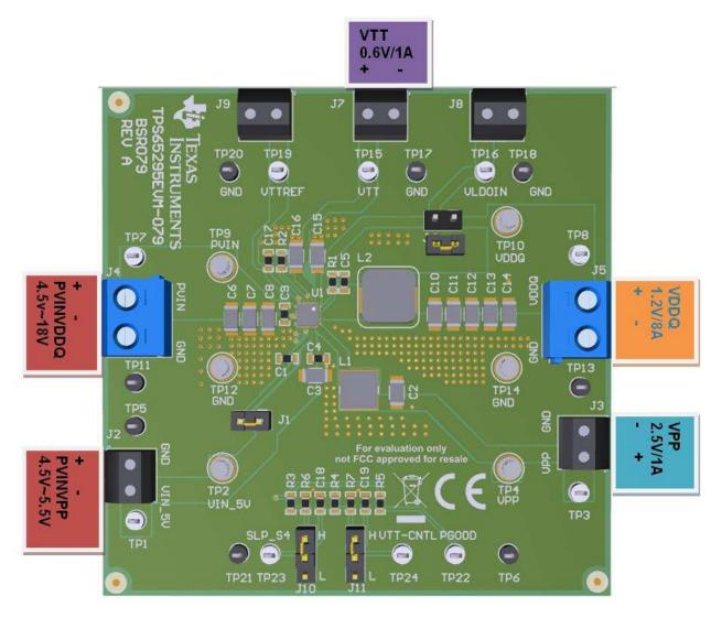
Figure 1. Headers Description and Jumper Placement
