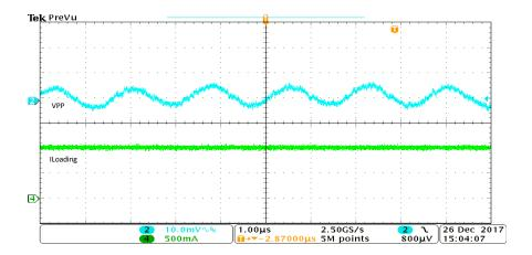
Figure 5. TPS65295EVM-079 VPP Ripple,  $I_{OUT} = 1 A$
