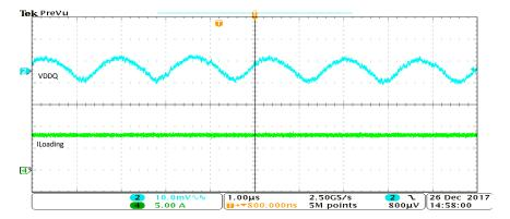
Figure 4. TPS65295EVM-079 VDDQ Ripple,  $I_{OUT} = 8 A$
