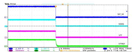
Figure 7. TPS65295EVM-079 Power Down Relative to SLP\_S4
